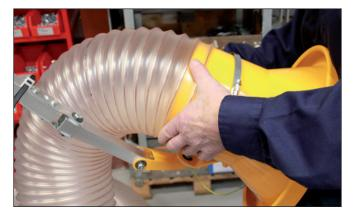
5. Attach the hose to the hood. Secure the hose to the hood using a clamp.
