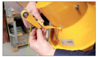
4. Now mount the hood on the outer joint by putting the supplied 8mm bolt though 3 spring washers, the hood bracket, the friction disc and secure with an 8mm lock nut.
