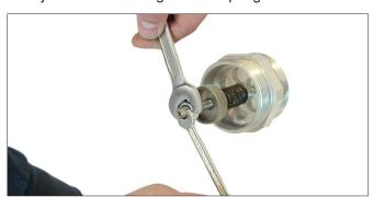
2. Then tighten the lock nut to secure the spring position.
