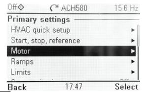
Setup the motor's rated current as indicated on the motor nameplate. For example 2.6A
