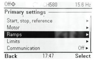
Setup ramp up time. Normally 20 seconds.
