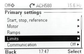
Setup minimum allowed frequency. Set at 15Hz. If set lower, both fan and inverter may suffer damage.
