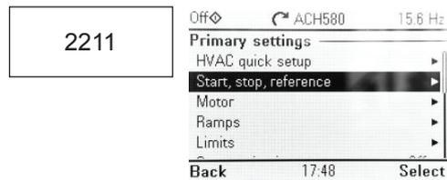
Setup the value(Hz) of max reference voltage(10V). If you set the parameter 2008 to ex. 55Hz then set this parameter to 55Hz too.
