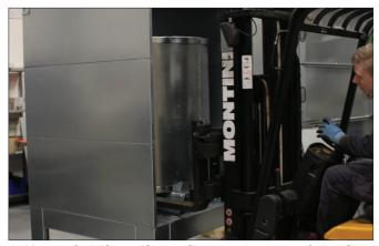
Use a forklift to lift the filter basket out of the filter cabinet.
