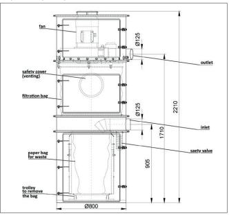
The unit consists of four modules which are connected together with tension bands:
