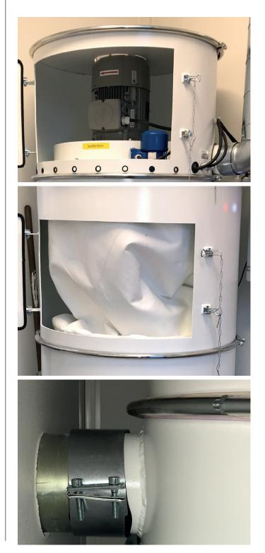
**Second top part** (picture in the middle above) Here is the suspension ring for filter and filter. The top two modules cannot be rotated relative to each other.
