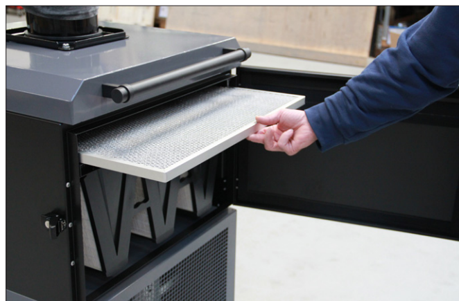
2. Take out the Alu mesh filter element
