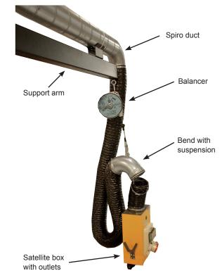
When mounting using bend and suspension a wire is placed in the hose to maintain a fixed distance between bend and satellite. Adjust distance as you wish.
