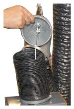
Suspension available after request. Shown here is a balancer, which will automatically pull the satellite back to its position after use.
