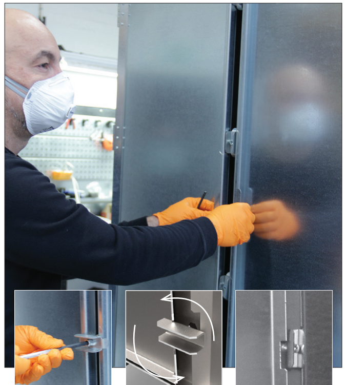
1. Loosen the bolts, turn the latch 90° to the left.
